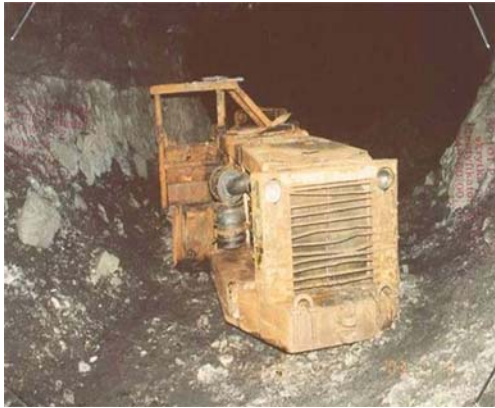
Figure 4: View of burnt LHD loader
